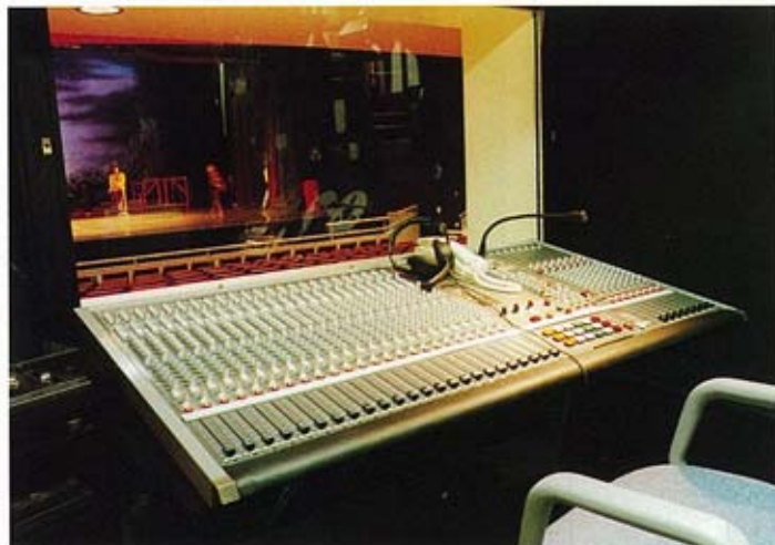
Allen & Heath's Saber Plus PA mixing console slightly modified for use at The Swan by Glantre.
