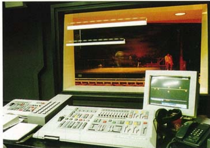
Compulite's Applause console in what was intended to be the projection room.
